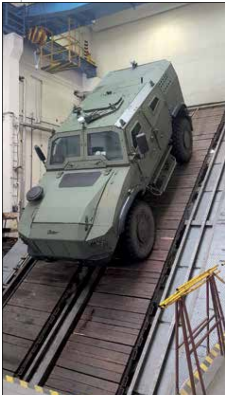
■ In testing the effectiveness of the parking brake system, the Gerlach achieved a slope of 83.9%.
