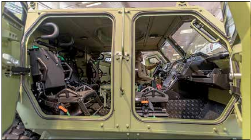
■ View into the Gerlach arranged in the standard 2 + 4 crew configuration.
