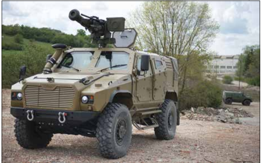
■ Virtually any weapons system up to 500 kg can be mounted on the vehicle roof
